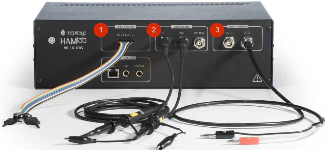
Logic analyzer probes (1), Oscilloscope probes (2), Signal generator connections (3)
