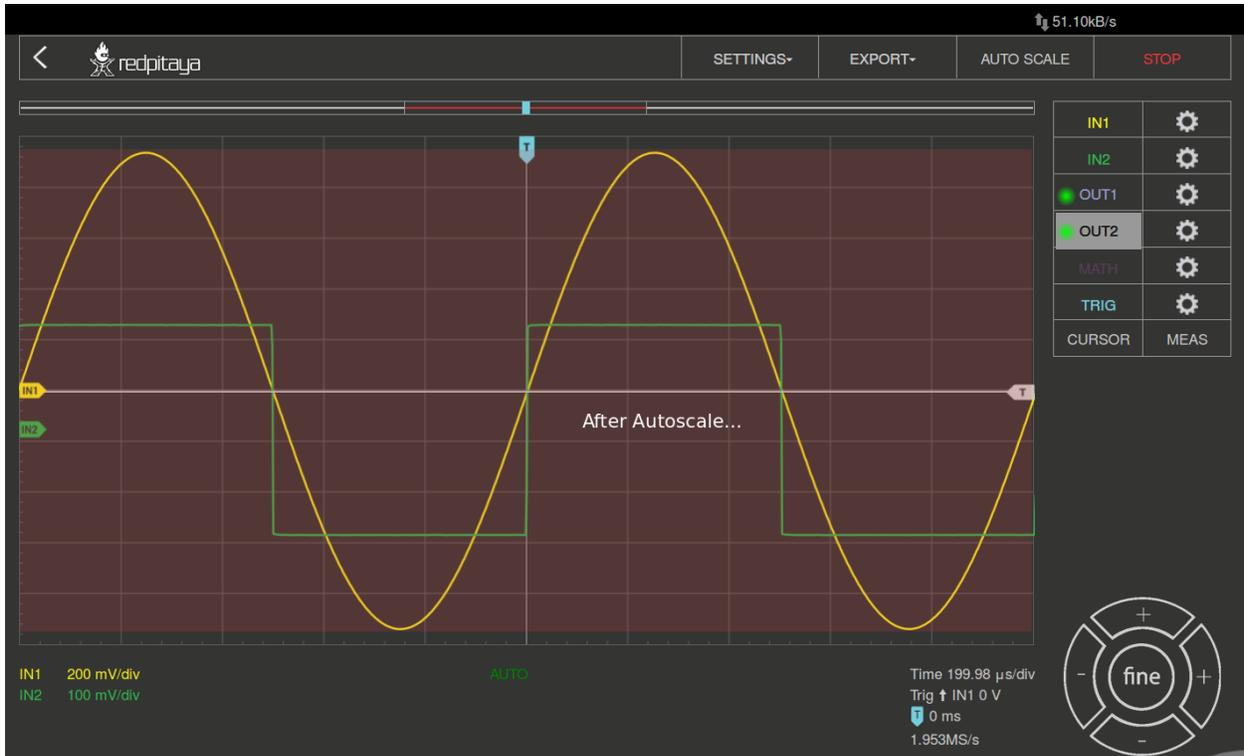
**INPUTS:** On the right side of the Oscilloscope&Sig. Generator application interface the IN1 and IN2 channels are listed. By a simple click on the name of a channel (not the gear) the channel gets highlighted and you can simply control all the settings of the respective channel.
