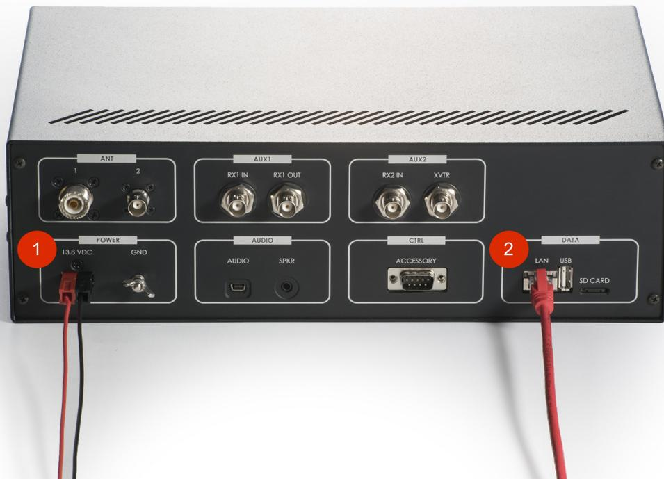
Anderson Power Pole™ power connector (1) Ethernet connection (2) - connect the HAMlab to your local network using ethernet cable.
