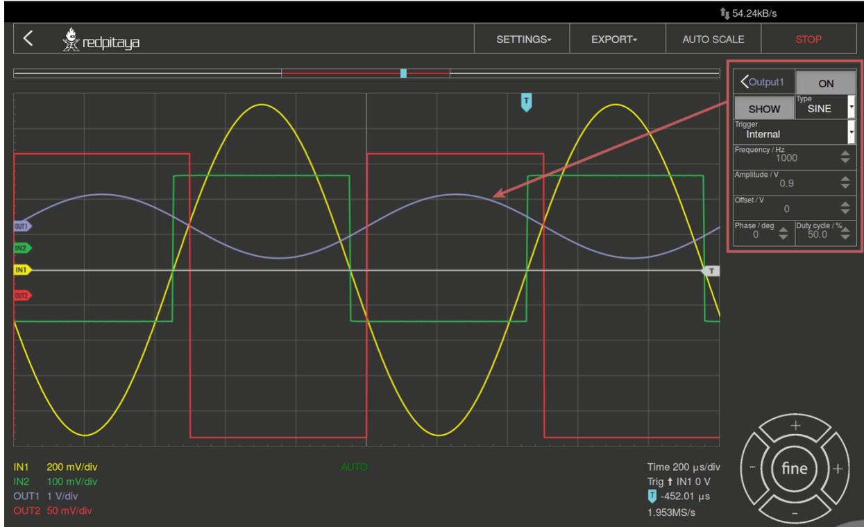
On the right side of the Oscilloscope & Sig. Generator application interface the **OUT1** and **OUT2** channels are listed.
